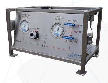
Trident Australia Gas Booster Unit incorporating a choice of Haskel AGT Series pumps available for pressures to 20,000 psi.
